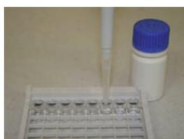
Add 100 microlitres of the Substrate Solution to each well.
