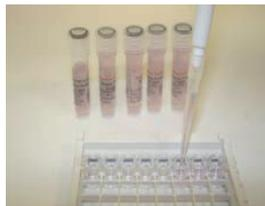
Add 100 microlitres of Standards and Samples to their allocated Antibody-coated wells.
